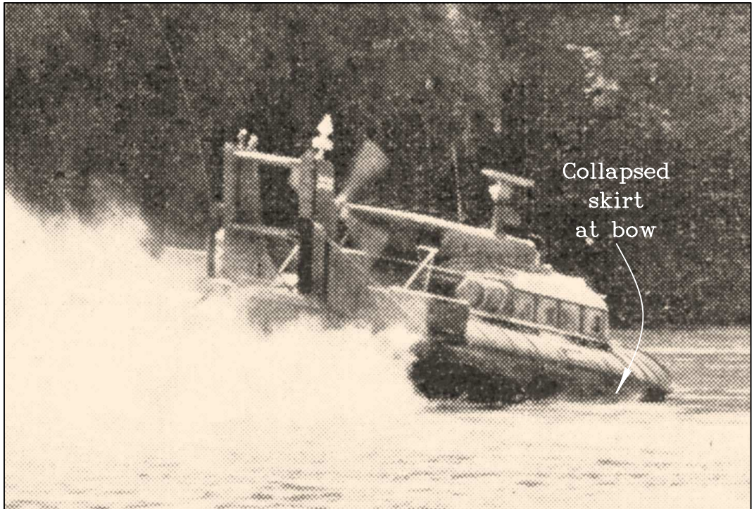
Figure 9.10: Plow-In of Jetted-Skirt Hovercraft (b) Plow-In Phenomenon
