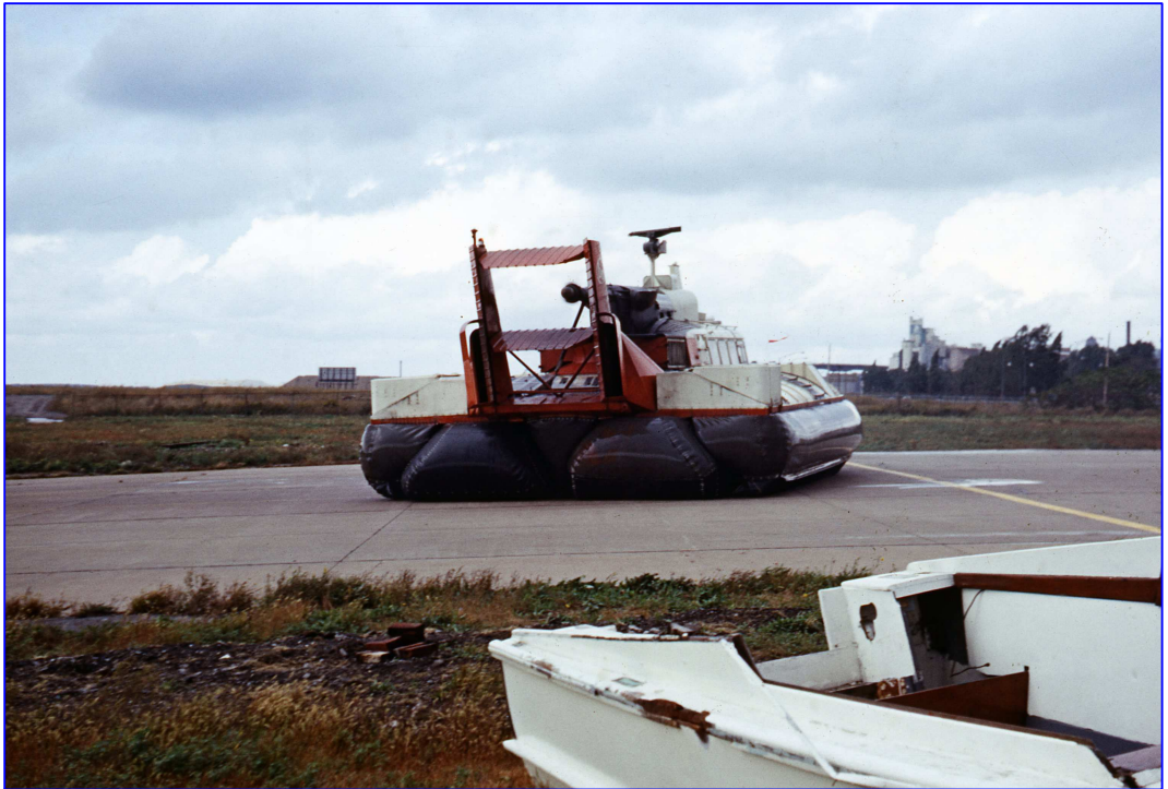
Figure 9.4: Stern and Rear Corners of Early Skirts (e) Saunders-Roe Ltd SR.N5 Hovercraft
