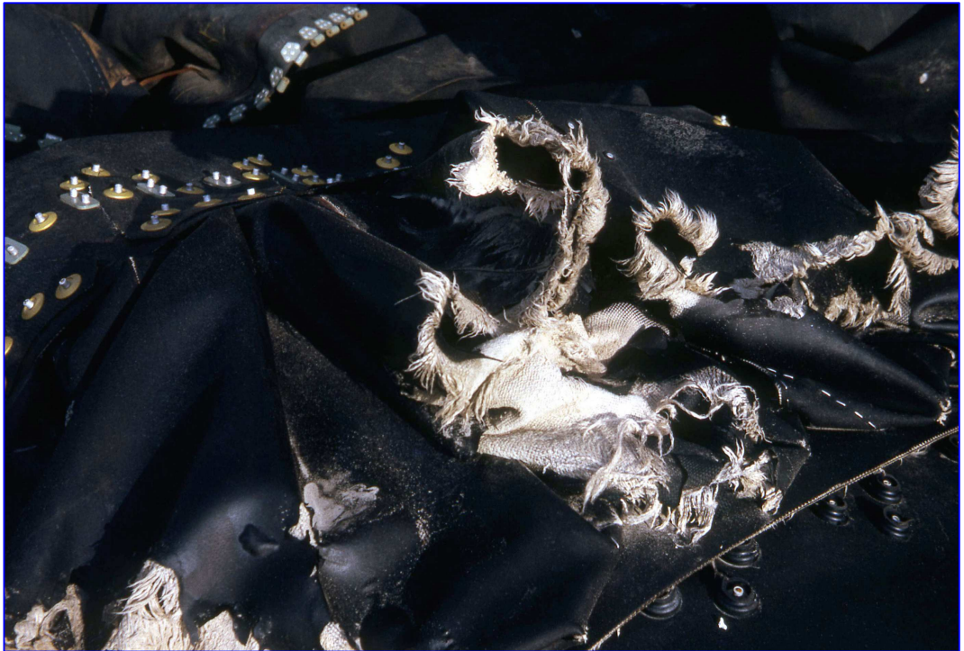
Figure 9.17: Miscellaneous Details of Air-Cushion-Vehicle Skirts (b) SR.N4 Worn Fingers
