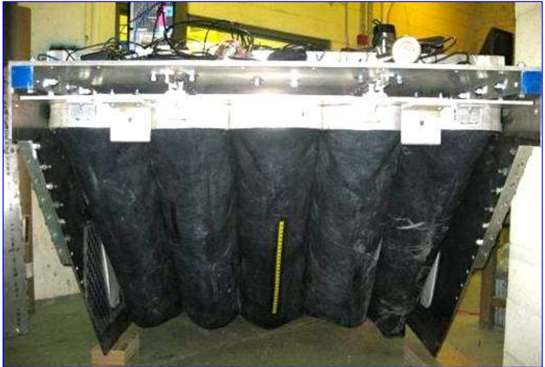
Figure 9.24: Apparatus for Testing a Bow Seal (d) Finger Seal
