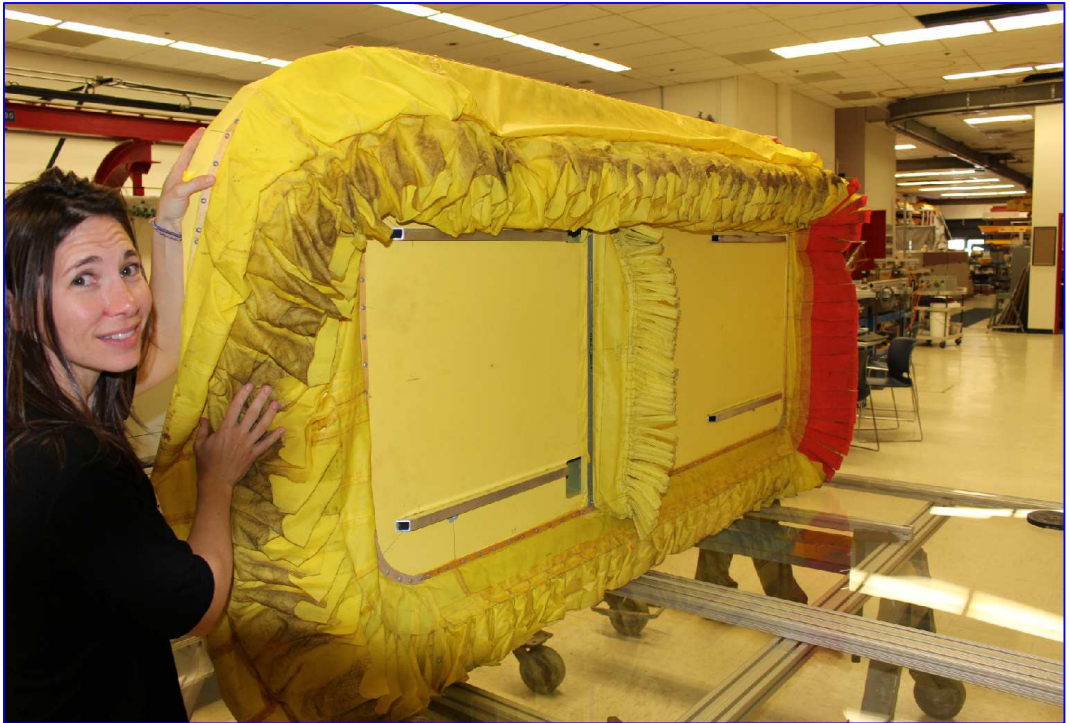
Figure 9.8: Finnish Navy T-2000-Class Tuuli (a) Skirt Platform
