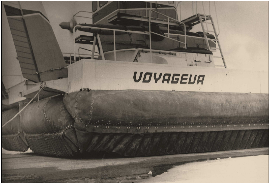
Figure 9.4: Stern and Rear Corners of Early Skirts (d) Textron Marine & Land Systems Voyageur Corner View
