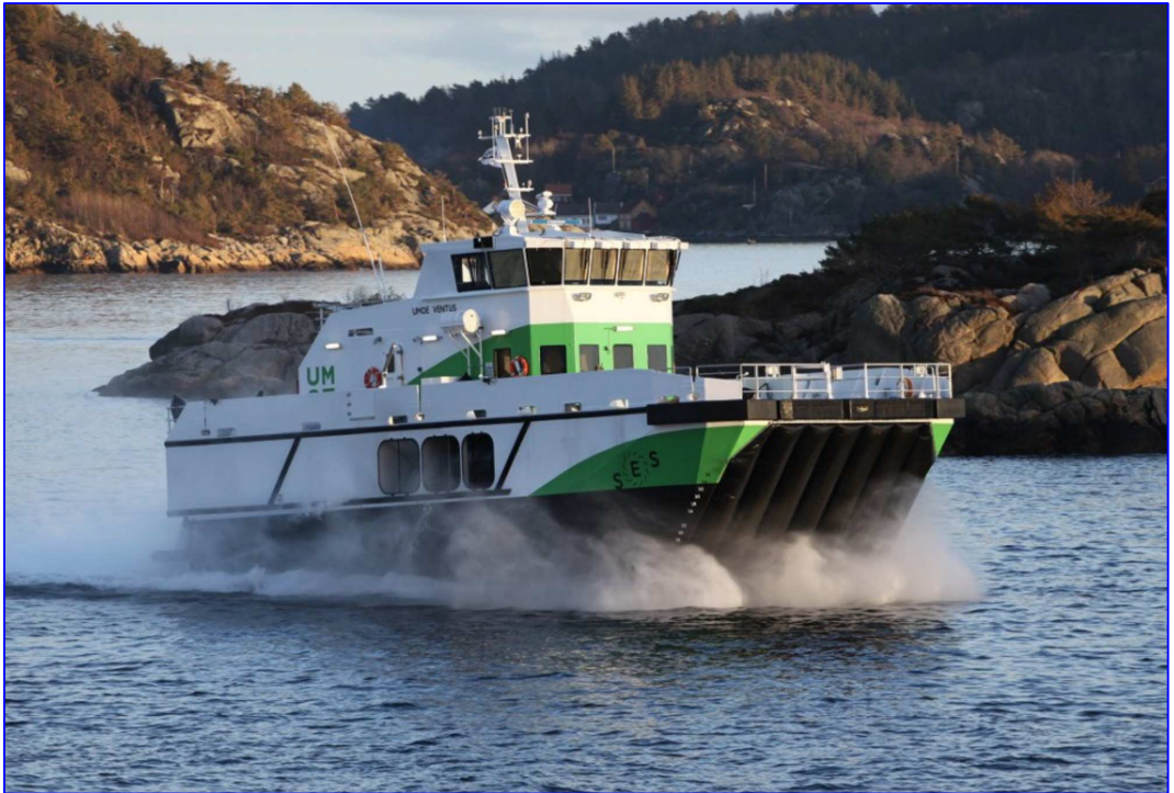
Figure 10.17: Umoe Mandel AS Surface-Effect-Ship WaveCraft (b) Prototype Craft Umoe Ventus at Speed
