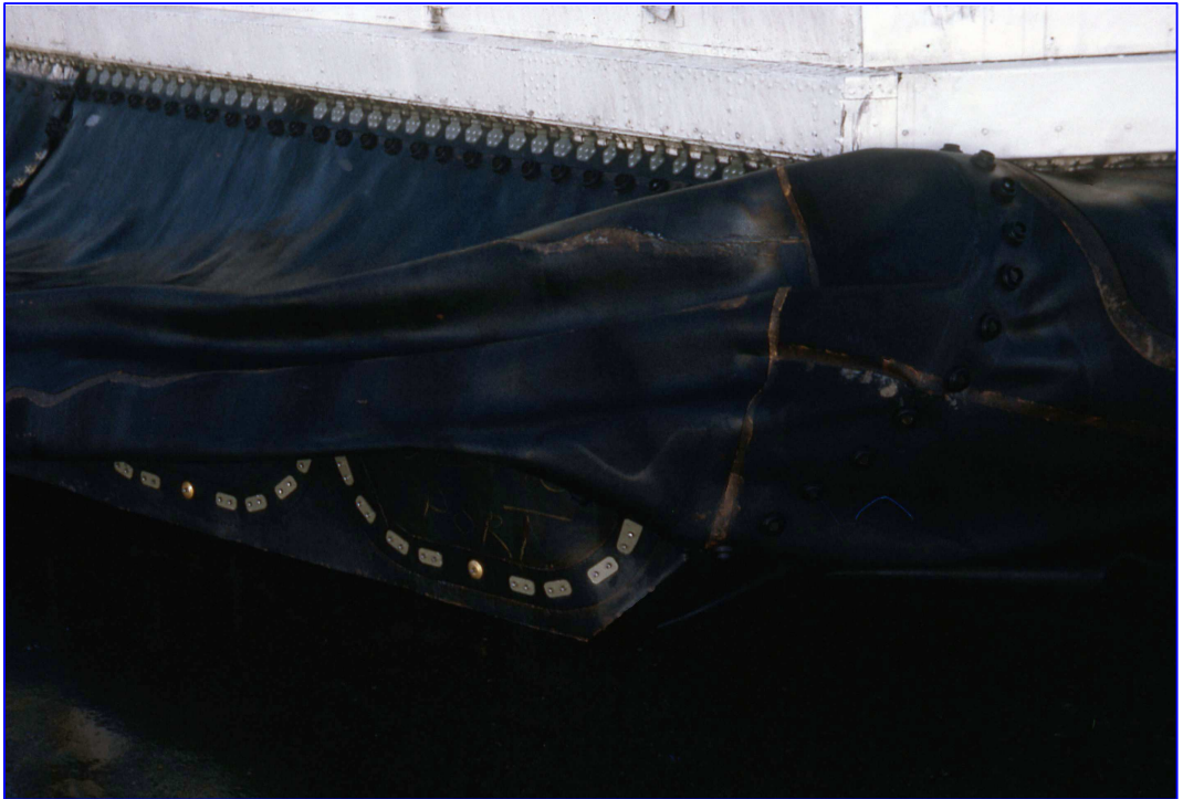
Figure 9.17: Miscellaneous Details of Air-Cushion-Vehicle Skirts (a) SR.N4 Finger Attachments
