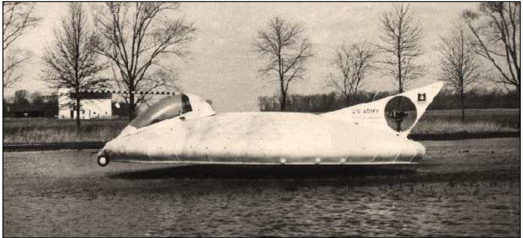
Figure 8.2: Early Air-Cushion Vehicles in the United States (c) Princeton University P-GEM over Water
