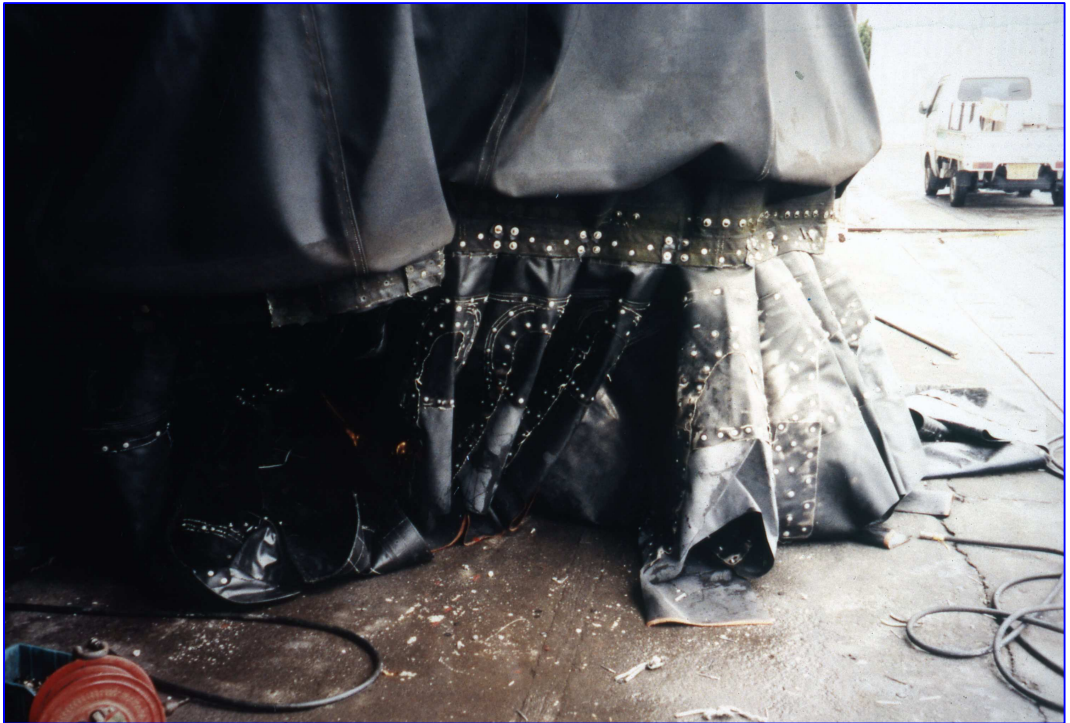
Figure 9.17: Miscellaneous Details of Air-Cushion-Vehicle Skirts (d) MV-PP10 Repaired Fingers
