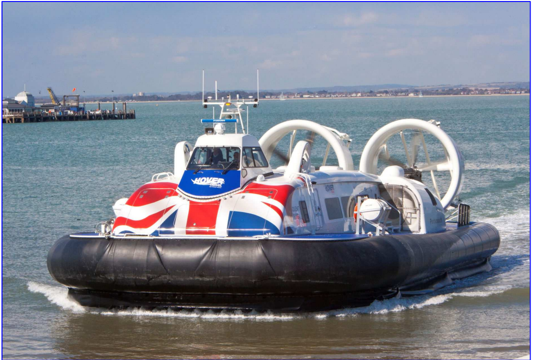
Figure 9.6: Tapered Skirts on Air-Cushion Vehicles (d) Griffon Hoverwork Ltd 12000TD
