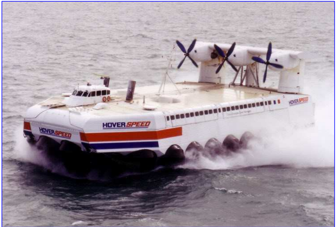
Figure 8.17: SEDAM N.300 and N.500 Naviplanes (e) N.500 with Widened Jupes over Water Ingénieur Jean Bertin
