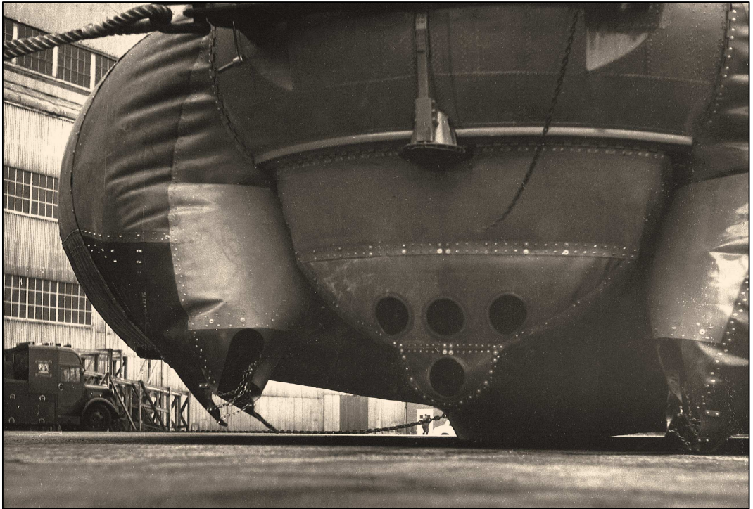
Figure 9.4: Stern and Rear Corners of Early Skirts (a) Saunders-Roe Ltd SR.N2 with 1.22-Meter Skirt
