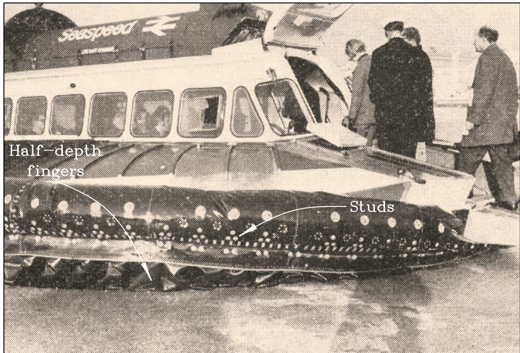
Figure 9.10: Plow-In of Jettied-Skirt Hovercraft (f) Fingers and Studs at Skirt Bow
