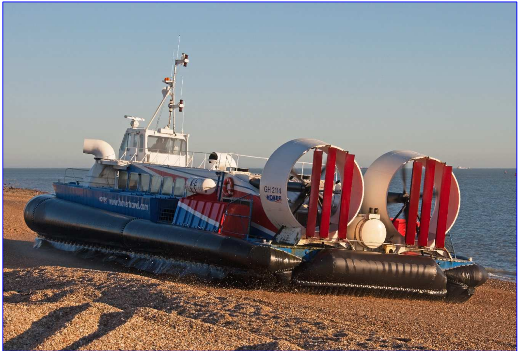
Figure 9.5: Stern and Rear Corners of Modern Skirts (c) British Hovercraft Corp. AP.1-88 Hovertravel Freedom 90
