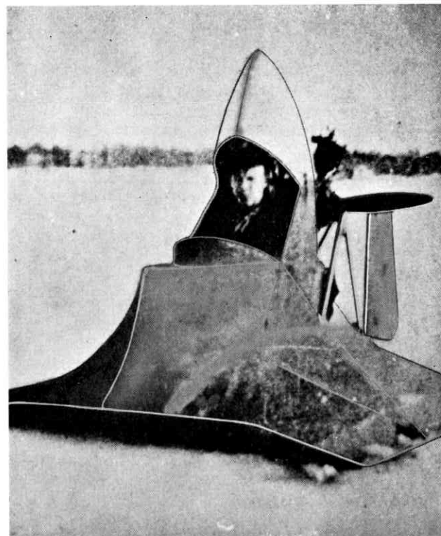
Figure 29. Kaario's first ground effect machine, built in Finland in 1935. It attained a speed of 12 knots with a 16 hp engine
