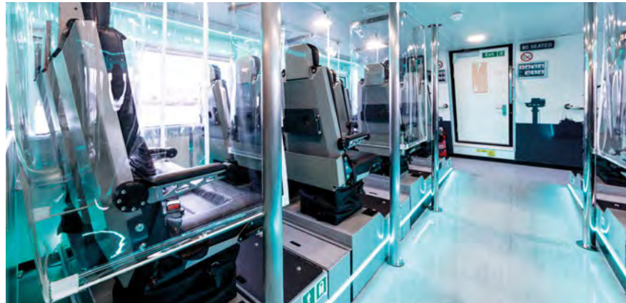
Plexiglas dividers were installed around CWind Pioneer's passenger seats in response to the COVID-19 pandemic
