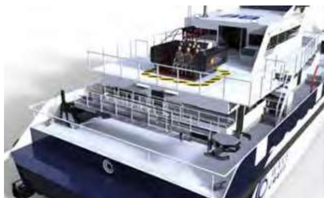
Figure 4: The Wavecraft Voyager 38's personnel transfer systems may include a motion-compensated gangway and SeaSpyder
