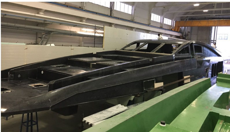
CARBONOVUS Azimut 115 deckhouse fabrication
