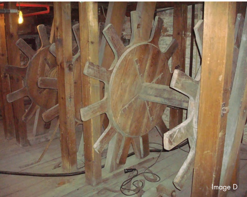
Image A: The lowest sub stage machinery with large drums and shafts. Image B: Fly loft with work bridges. Image C: Upper level fly loft. Image D: Winches below the stage. Image E: Chariots of the highest sub stage level.
