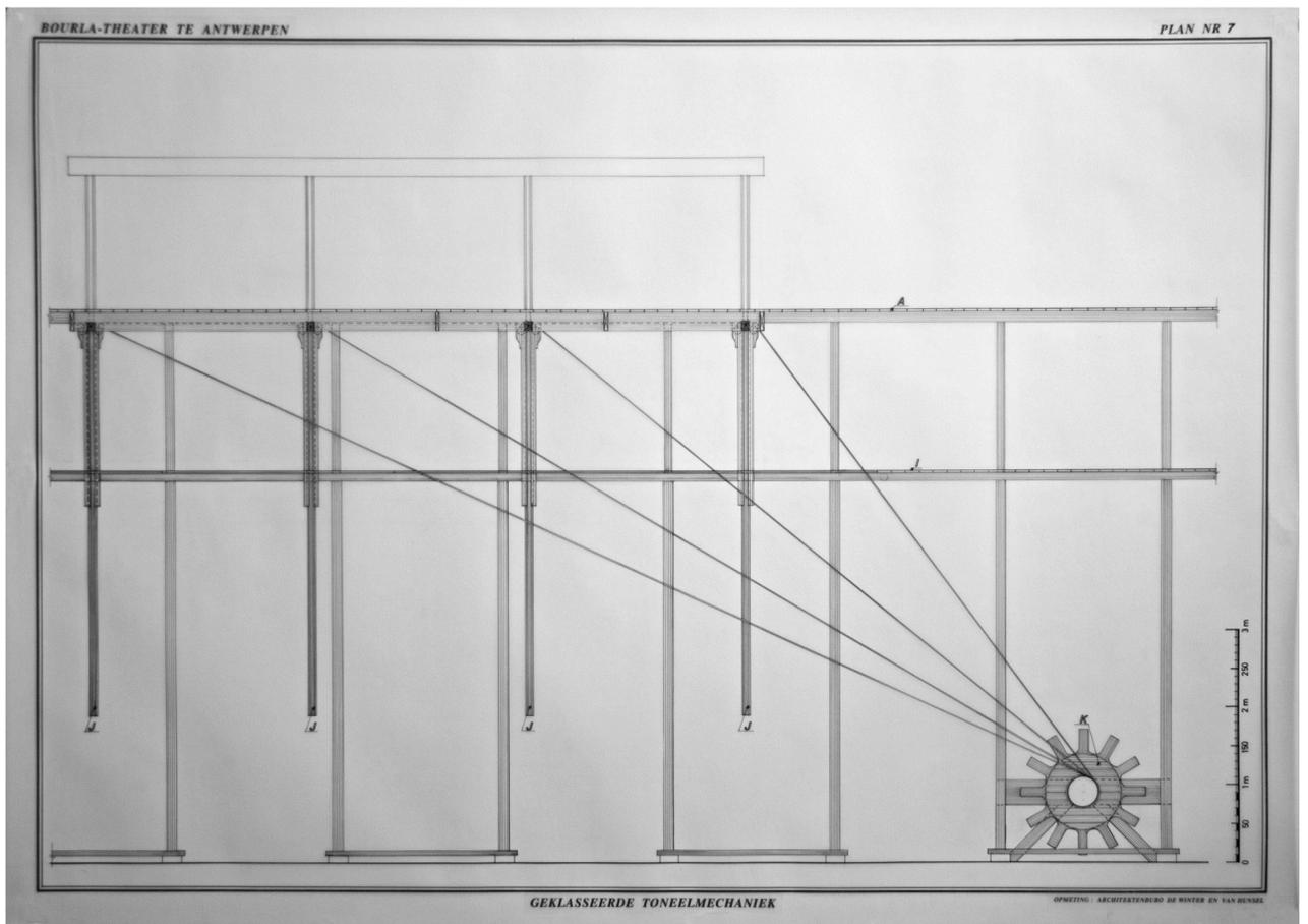
connected that runs into a slit along the batten. The cassette contains sheaves that change the direction of the rope in order to manipulate the height of the batten and to connect counterweights.
