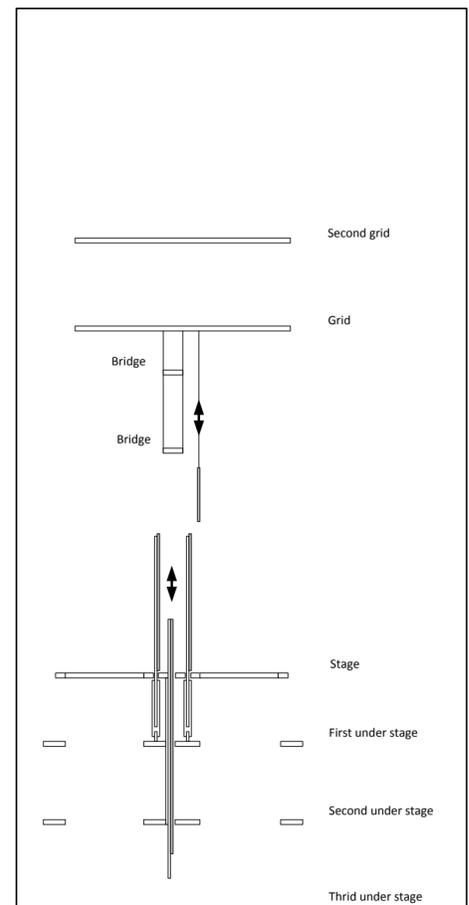
blocks on the outside, go up and down. On the inner (stage) side, pin rails are placed to fix ropes coming from the head blocks on the grid. Additional winches are placed on different points to be able to pull up the counter weights.
