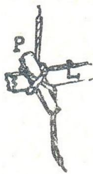
to be fixed can be connected to the rail by tying them off (with a specific knot). If a loose pin rail is used, the pins can be retracted to release the rope. In some cases, a double pin rail is used, the lowest position can stay fixed.
