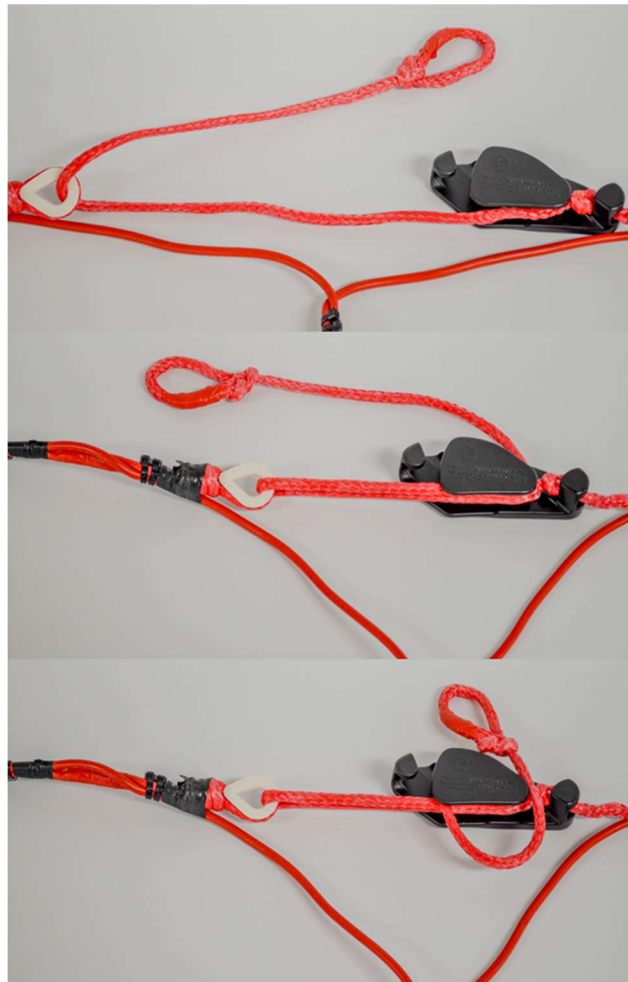
Figure 7. How to operate a cleat. In the beginning the rope is loose (top), bring the rope beneath the black cleat and towards up and tighten it (middle). After lock the rope by bringing it downwards to the left side of the black cleat (bottom).
