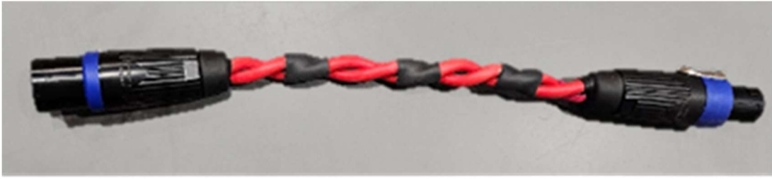
Figure 8. Tx coil adapter for Multiturn Tx coils (333 or 443).
