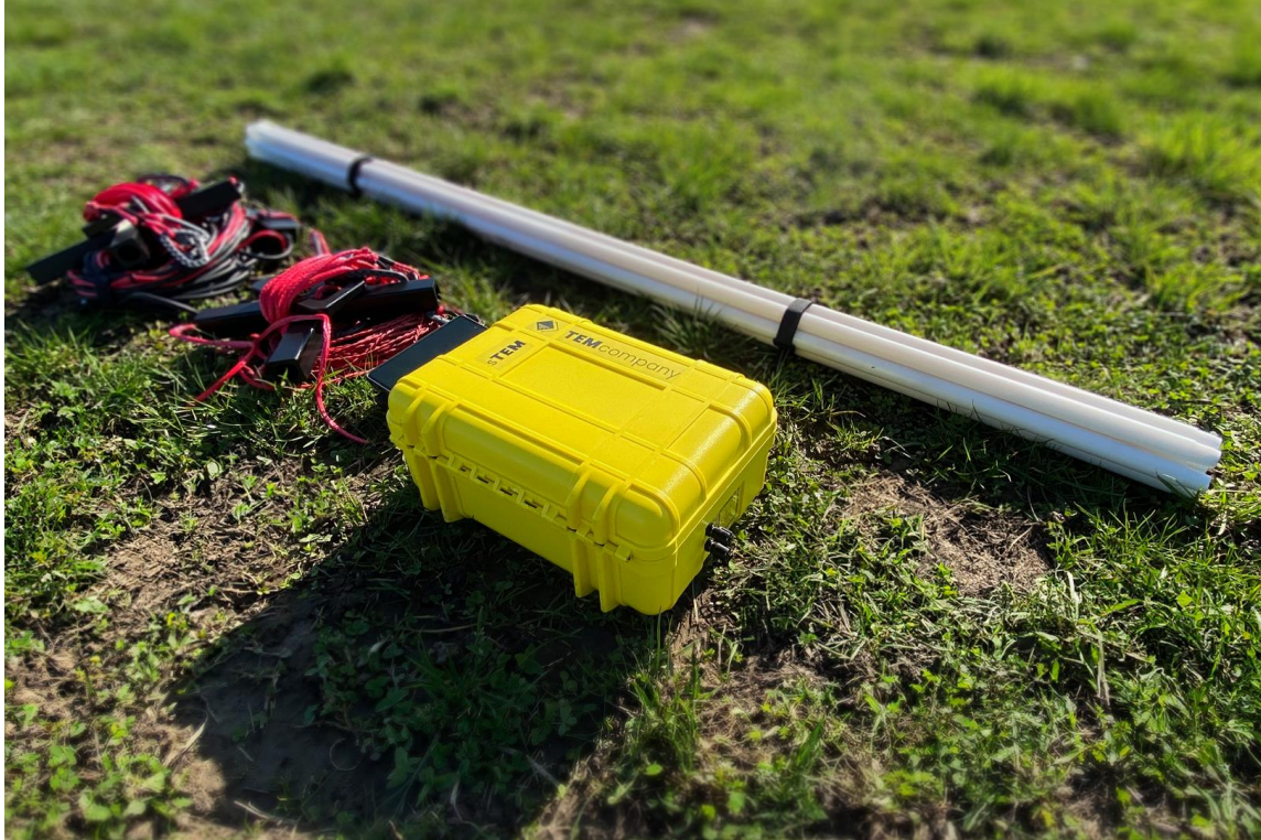
Figure 3: The picture shows the sTEMprofiler system. The yellow box is the sTEM instrument, the white rods are used to build the rig and the black and red cables to the left is the receiver and transmitter coils.
