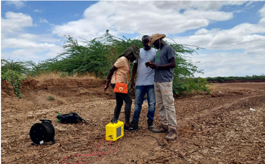
Figure 1 The sTEM system in operation. The system is operated from an Android or IOS app.
