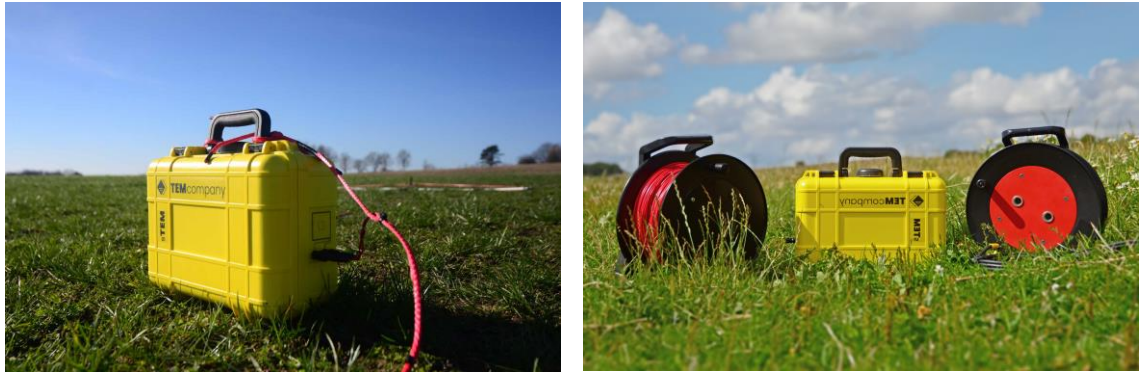
Figure 3 the picture shows the sTEM unit and the transmitter and receiver drums.
