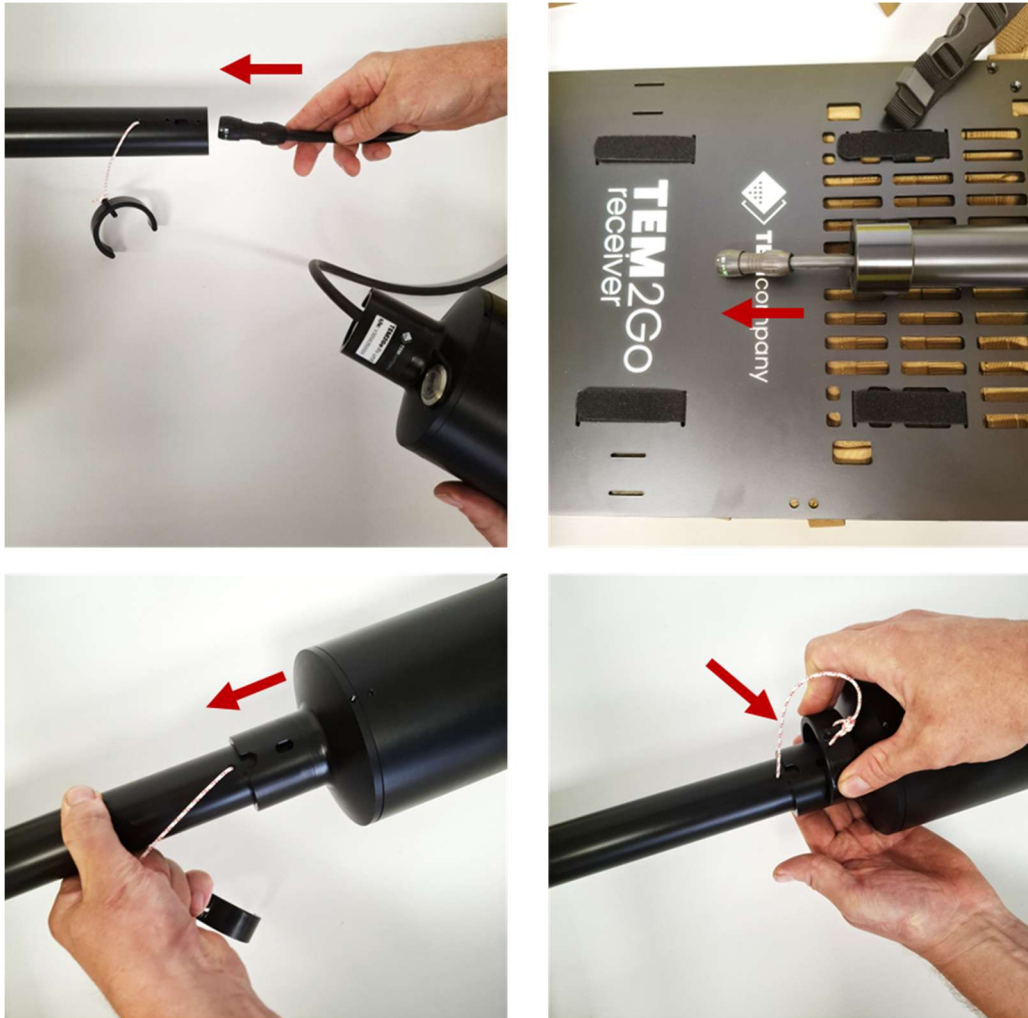
Figure 15: Mounting the Rx unit on the receiver backpack. Insert the pole in the bracket (left), add the Rx unit on top (middle) and secure everything with the provided clips (right).
