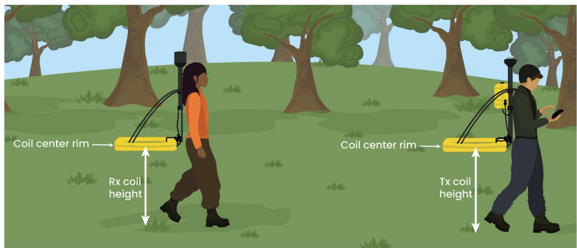
Figure 24: Depiction of proper coil height measurement
