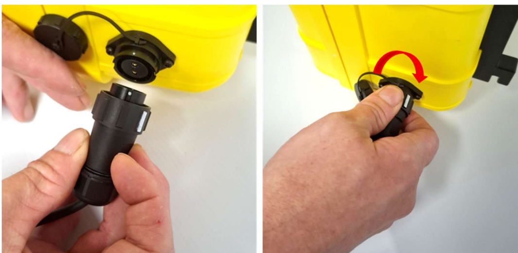
Figure 19: How to plug in the connector to the Tx unit.
