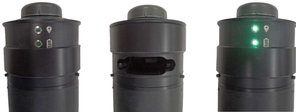
Figure 8: Steps to power the receiver unit. After inserting the battery and pressing the power button, the two LED lights turn on.
