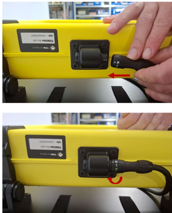
Figure 16: How to connect the Rx unit cable to the connector on the Rx coil.
