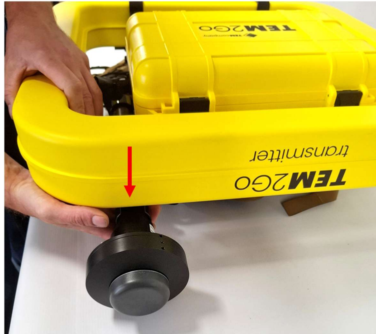
Figure 22: How to secure the Tx coil to the pole on the transmitter backpack
