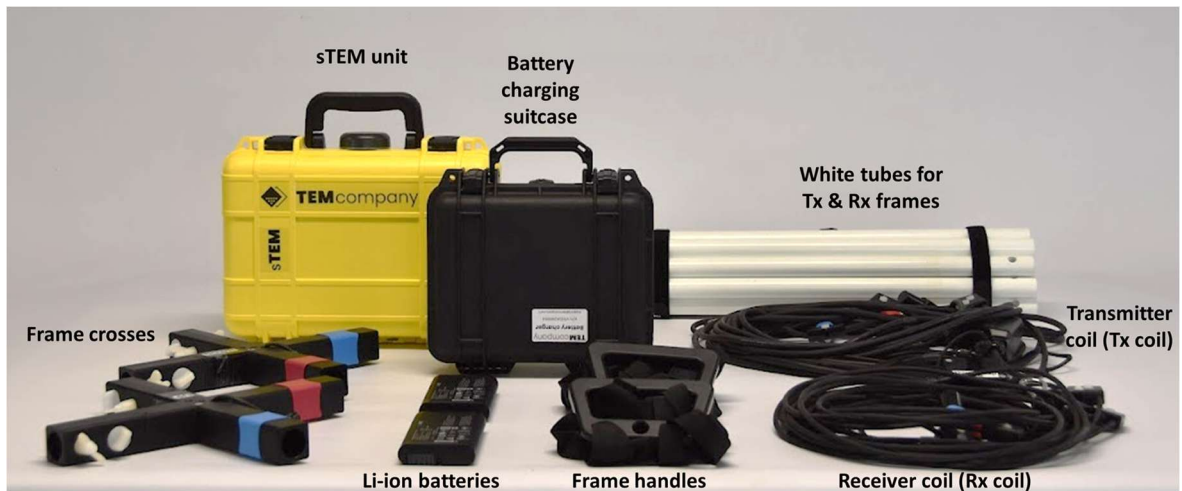
Figure 10. Main components of the sTEM profiler system. The total system weight for a sTEM profiler setup including sTEM unit is approximately 19.5 kg (43 lbs) (excl. battery charging suitcase).
