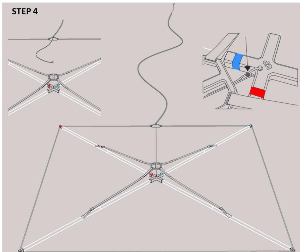
Figure 14. Clipping in towing safety ropes.
