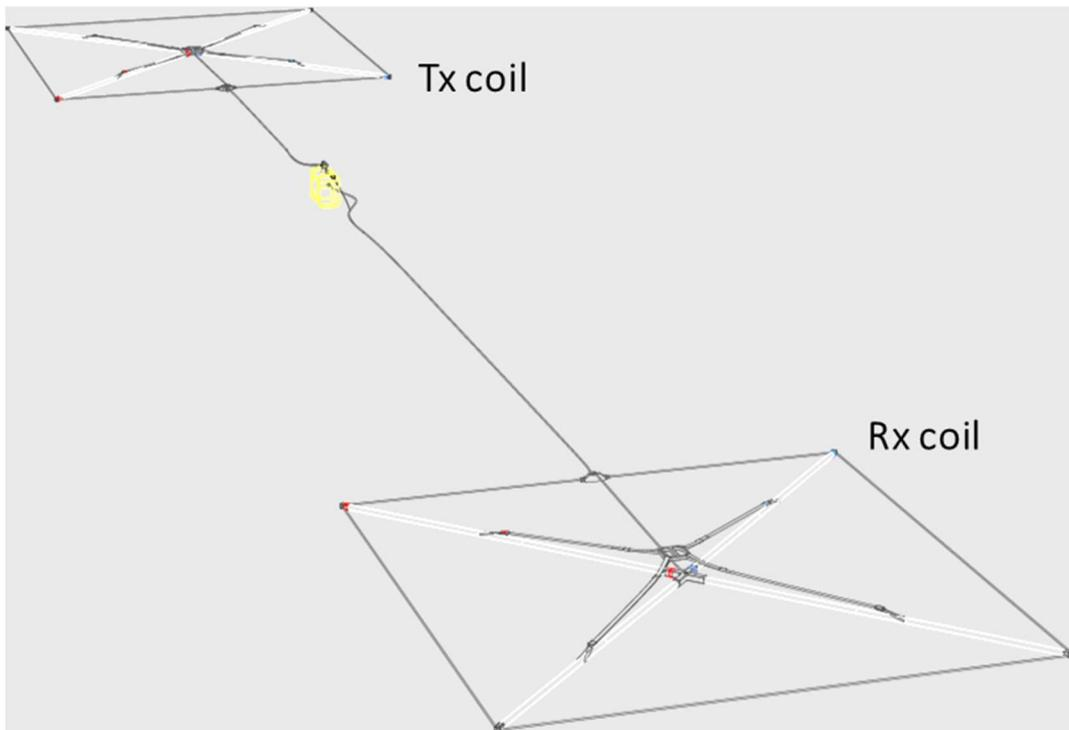
Figure 16. Fully assembled sTEM profiler system.
