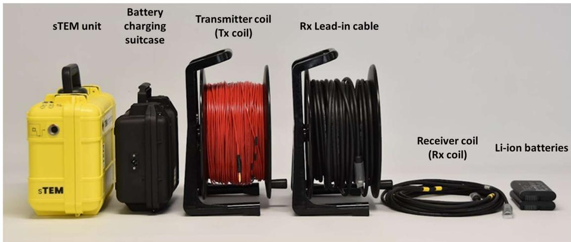
Figure 3. Main components of the sTEM system
