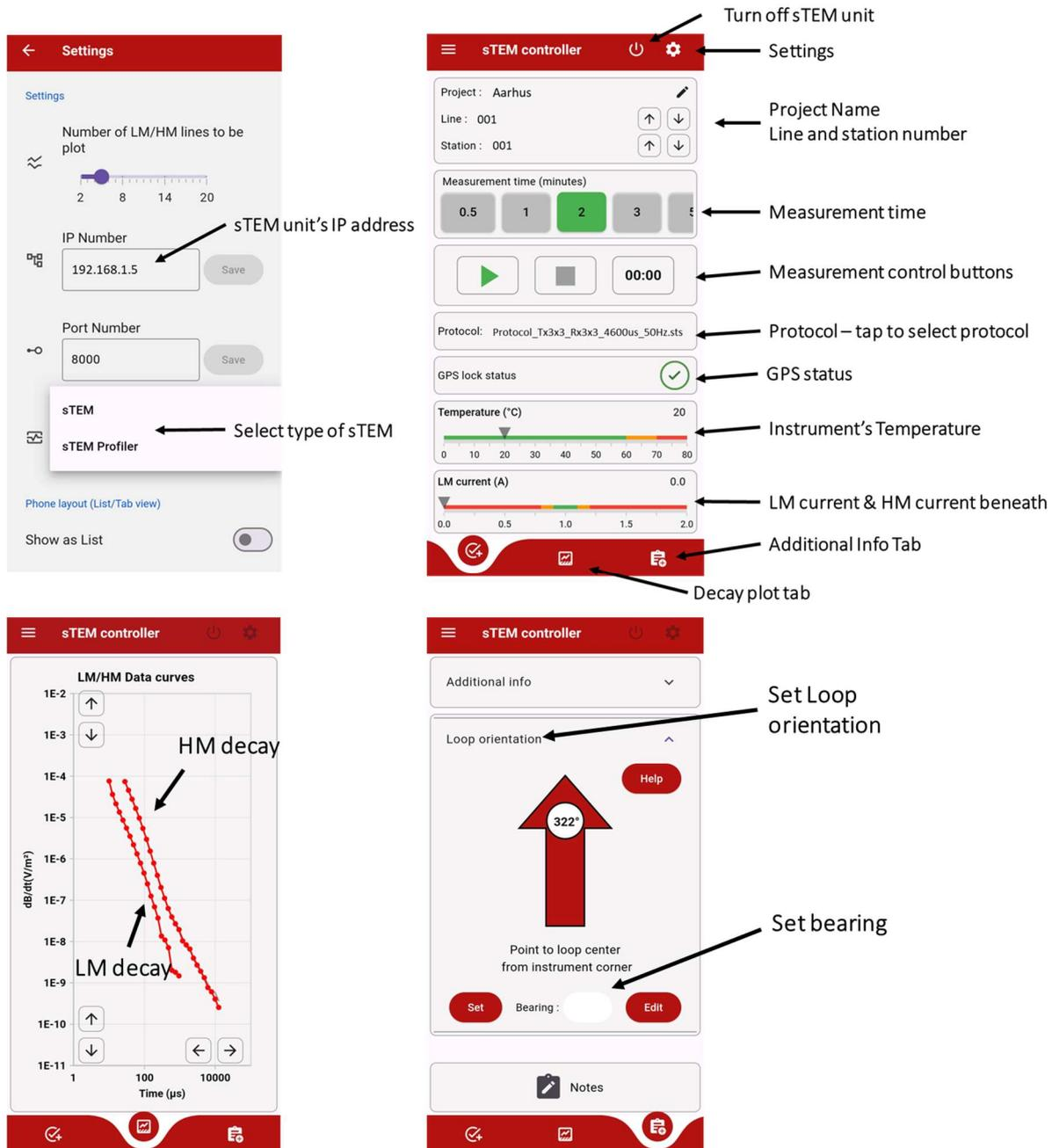
Figure 18. sTEM Controller app environment. Version 1.1.0.
