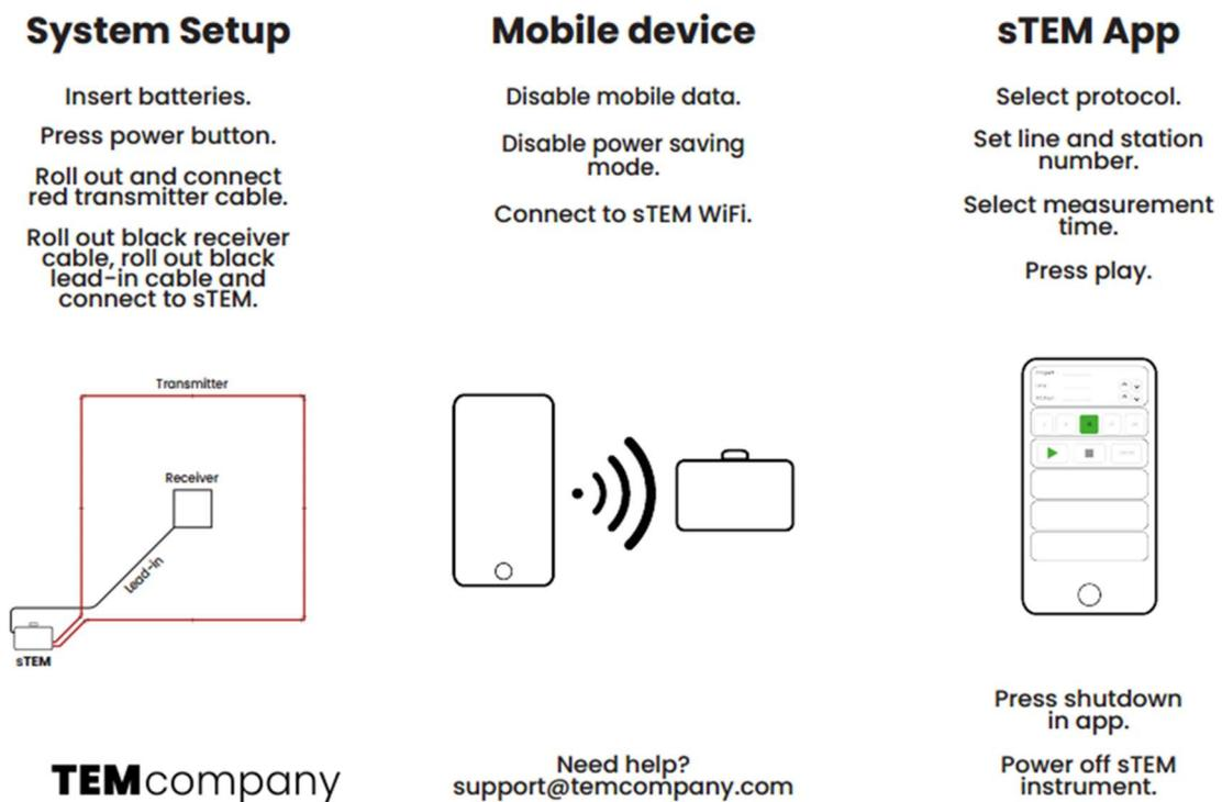
Figure 1. Quick sTEM operation guide
