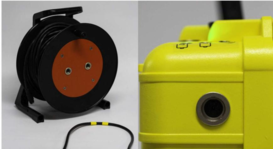
Figure 10. Lead-in cable drum (left) with connectors for receiver cable. Yellow marking showing the meeting point between lead-in cable and Tx coil.
