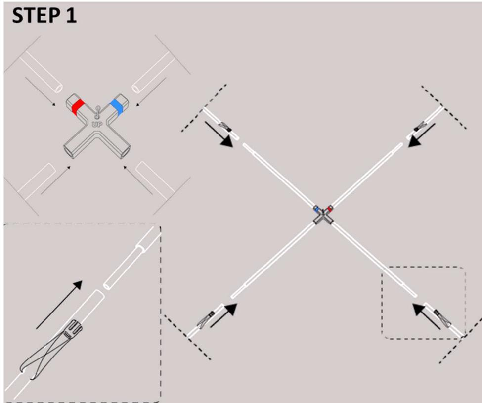
Figure 11. Assembling rods into center piece.
