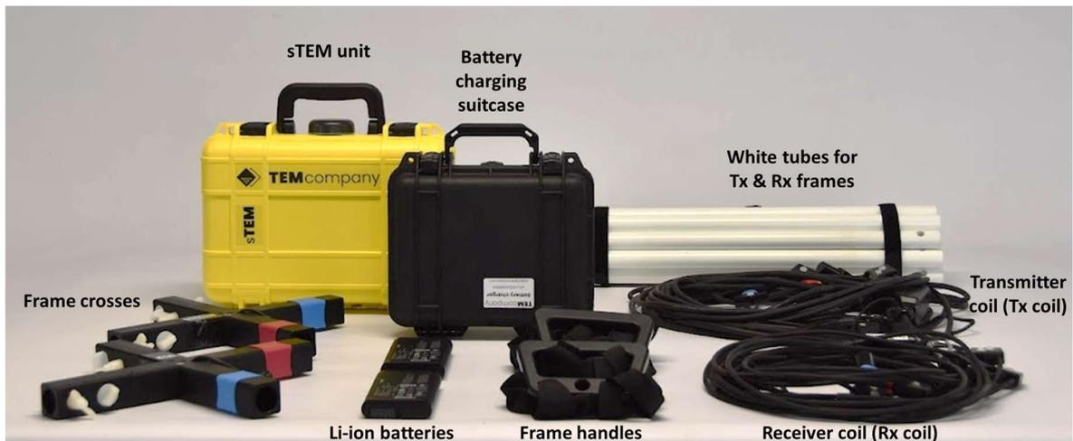
Figure 4. Main components of the sTEM profiler system, The total system weight for a sTEM profiler setup including sTEM unit is approximately 19.5 kg (excl. battery charging suitcase).
