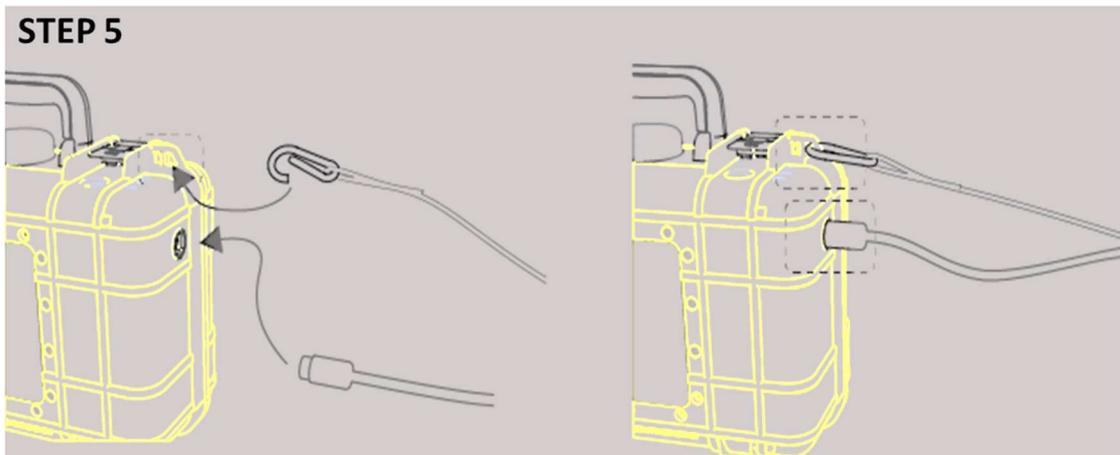
Figure 15. Connecting to sTEM instrument.
