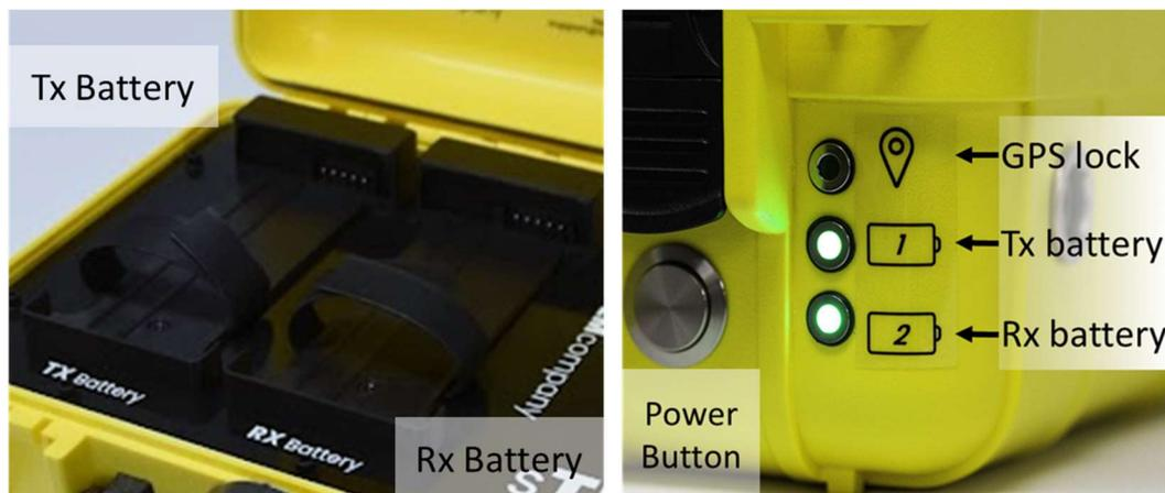
Figure 5. sTEM unit. Battery slots and battery LED lights when batteries are inserted.
