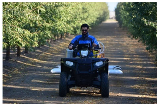
Figure 2. Collecting tTEM data in the orchards.
