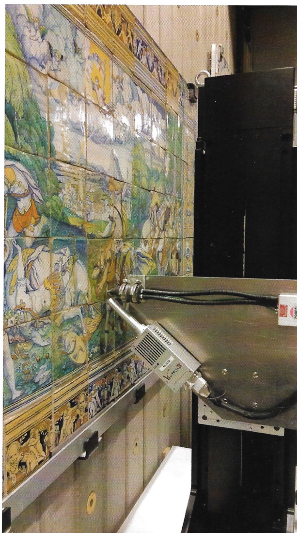
Figure 7. Scanning of the tile panel by the AXES Research Group in the MASiVisible Storage before restoration (2015) (Copyright Geert Van der Snickt, AXES Research Group, University of Antwerp)
