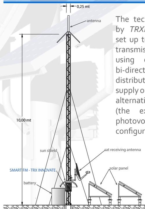
The technology developed by *TRXInnovate* allows to set up totally self-sufficient transmission stations by using either mono- or bi-directional satellite distribution, with a power supply obtained by means of alternative energy sources (the example shows a photovoltaic panel + battery configuration).
