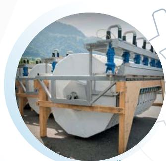
Disk filter unit on transport frame
