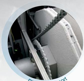
Disk filter support system & non-metallic drive chain
