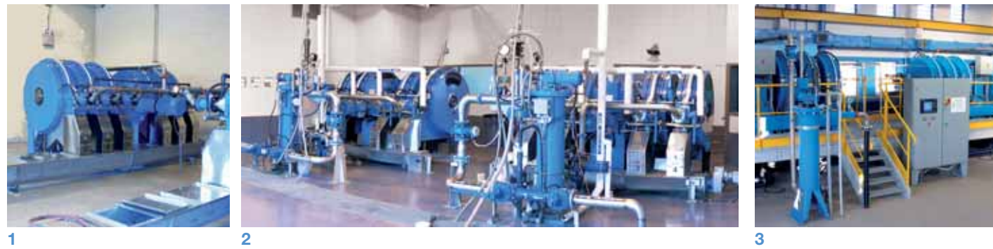
1 Charleston Plum Island Waste Water Treatment Plant (136 million litres/day) [USA]. Two 6-channels equipments. On-site testing was carried out using different technologies, leading to an objective context-specific assessment between the rotary press and well-known centrifuge brands. Based on cost, operation and maintenance and monitoring requirements analysis, the rotary press was adopted as the main dewatering equipment, to replace existing ageing equipments.
