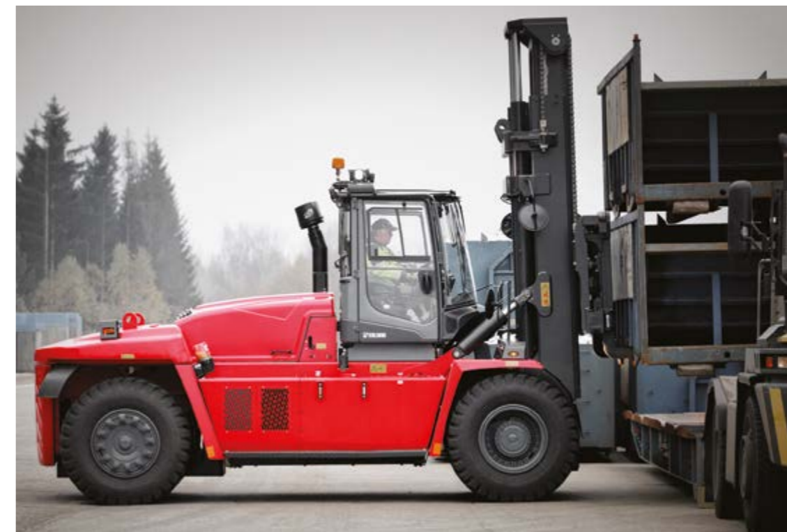
BELOW: At 300mm lower, the carriage of the DCG180-250 models further improves visibility in the forward direction
