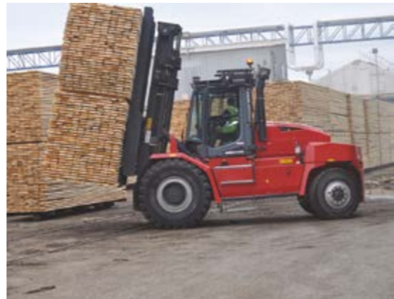
MAIN IMAGE: Larger-than-usual (23.5in) tires on the Kessler drive axle act like suspension to enhance operator comfort
