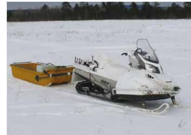
BELOW: Defence R&D Canada sponsored this Mogile Technologies research project, dubbed Loki (pronounced ‘low key’). It can run with a conventional petrol engine and switch to electric when required. Simon Ouellette says, “The military were primarily interested in the acoustics of the vehicle, and with a quiet drivetrain, this was easier to study”
