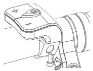
5. Link the male connector at the display with the female connector at the EB-BUS.
