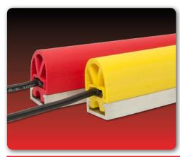
The TS-26 Sensing Edge is a general-purpose, medium profile, pressure-sensitive edge. It provides minimum compliance before activation, and about 3/8 inch of overtravel cushioning after activation. This product is excellent for applications requiring side activation. TS-26 Edges are available in two mounting configurations: snap-in channel-mount (flat or angle), clamp-mount.
