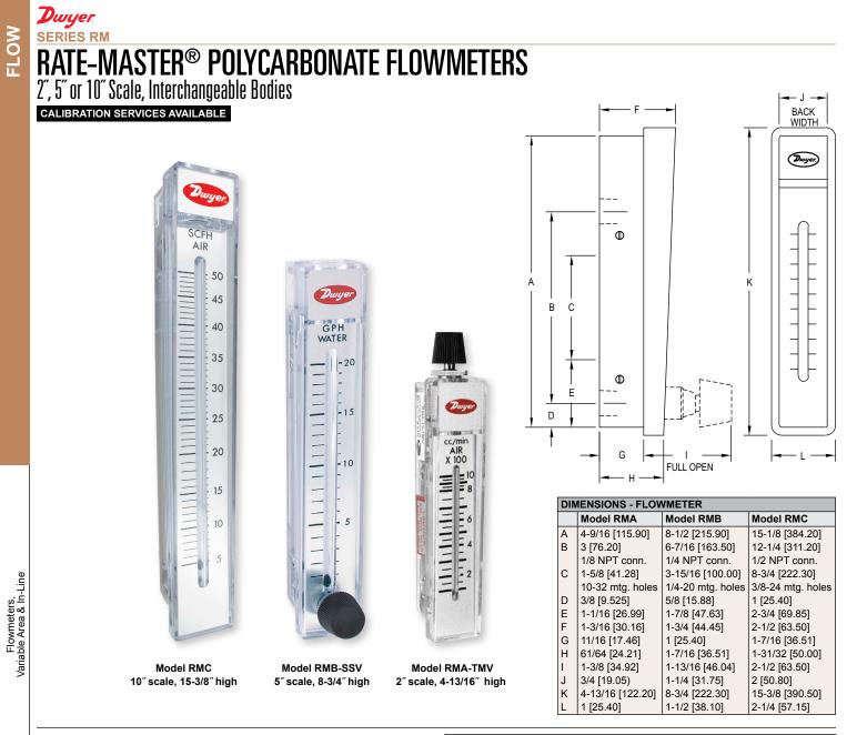
The **Series RM Rate-Master® Polycarbonate Flowmeters** are a line of general use, direct reading precision flowmeters suitable for both gas and liquid applications. This Series consists of 2" (51 mm), 5" (127 mm) and 10" (254 mm) scales that can be panel or surface mounted with optional precision metering valves. Within a given Series, the Rate-Master® flowmeter bodies can be instantly interchanged, allowing the piping to remain undisturbed, interchangeability of the ranges, and easy cleaning.
