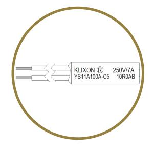
The YS11 can be used for on-winding and outside of resin packed motors by clamping or insertion. Since the YS11 has a plastic case, it does not need to be insulated from metal part of the motor.
