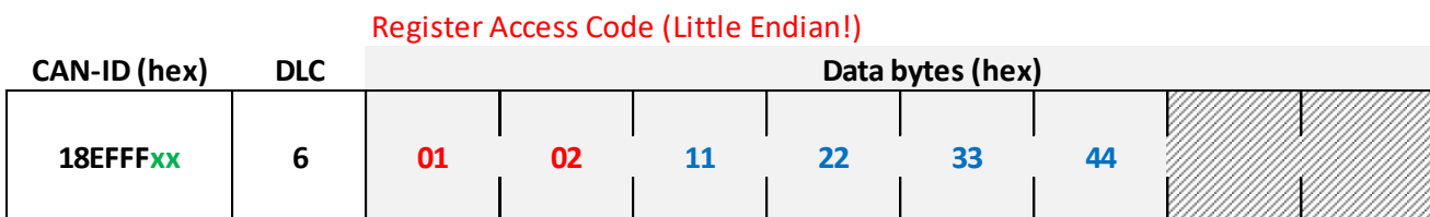
xx stands for the transducer's address Read Value 0x44332211 (in this case int32; Little Endian)
