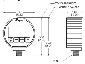
The **SERIES DPG-000** Digital Pressure Gage has a precise ±0.50% full scale accuracy. The 4 digit digital display will reduce the potential for errors in readings by eliminating parallax error commonly produced with analog gages.
