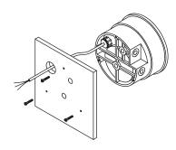
**B. SURFACE MOUNTING:** Drill (3) 3/16" dia. holes for mounting screws and (1) 7/8" dia. hole for wire assembly as shown in hole location drawing. Insert screws from rear of panel and thread into tapped holes on back of Photohelic® Switch/Gage case. If rear pressure connections are to be used, make 1/2" dia. holes located as shown in hole location drawing in left column.
