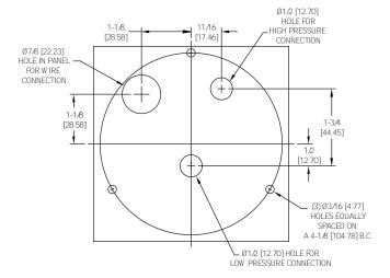
MOUNTING: The Photohelic® Switch/Gage may be either panel mounted or surface mounted.
