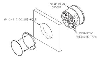
**A. PANEL MOUNTING:** Cut a 4-3/4" or 120mm dia. hole in panel and insert the complete unit from the front. Slip on the mounting ring and install the split snap ring in the groove on the bezel. Seat the mounting ring against the snap ring and thread the four screws through the tapped holes. Tighten screws against rear of panel.
