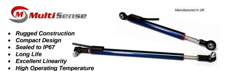
The MS-94 series of linear potentiometers are designed to withstand the harsh environments of motorsport, testing and industrial applications. Using proven 'Conductive Plastic' technology, the sensors offer high performance and reliability at operational temperatures up to +175°C
