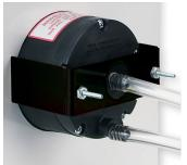
Mounting hardware is supplied with the Minihelic<sup>®</sup> II gage for panel mounting through a single hole, 2-5/8" (67 mm) in diameter. Panel thickness up to 1/2" (13 mm) can be accommodated with the hardware supplied. If necessary, surface mounting of the gage can be accomplished by means of two 4-40 screws into the tapped mounting bracket stud holes in the rear of the gage. Surface mounting requires clearance holes in the panel for the two pressure taps.
