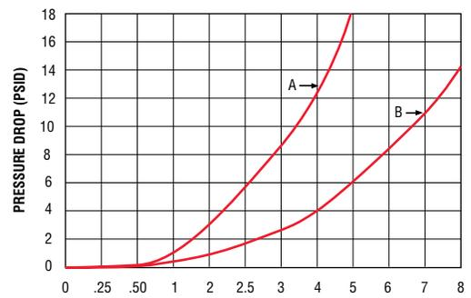
Tests conducted with water flow at 68°F (20°C).
