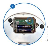
Activate Direct Pairing by pressing button under FS3 battery cover for 3 seconds – Buzzer and LED is activated.
