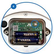
Confirm pairing by pressing button under FS3 battery cover.
