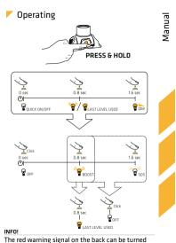
off/on by holding the switch ≥ 2.4 sec. in ON-Mode
