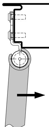
5. Adjust the lower hinge part welded on the frame. Pay attention to the correct use according to the marking on the hinge alignment tool for the respective hinge type («weld-on hinge» for weld-on hinges and screw-on hinges, «barrel hinge» for barrel hinges). Reach the desired adjustment by gently pushing or pulling.
