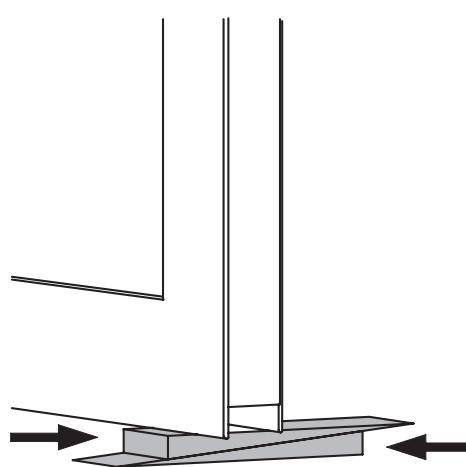
3. Open the door leaf approximately 10-20° and relieve the upper hinge e.g. by placing wooden wedges under the door leaf.
