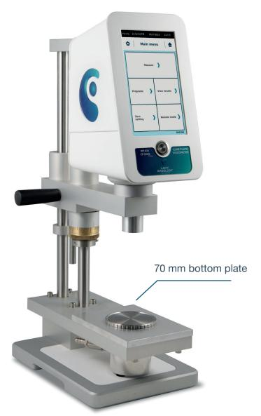
Equipped with a fluid circulation for temperature control (bath not included), the RM100 CP1000 PLUS will allow you to perform cone-plate and beaker measurements using the MS RV, MS VANE or MS KREBS mobiles.
