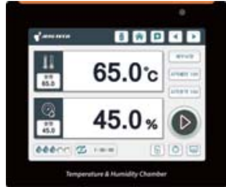
Large LCD touch screen controller (5.6 inches)
