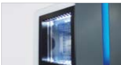
Tempered glass window with wire heater and LED lamp.
