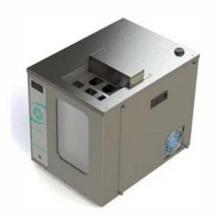
A five-button control pad on the EVS provides single step access to menus. The user interface includes selection of set-point, reference temperature (offset), units (°C, °F) and the chiller set-point.
