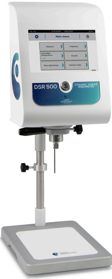
The rheometer with imposed shear rate equipped with a 7" touch screen to display the curves directly. And with direct report editing on a desktop printer, measuring viscosity or yield point has never been so easy!
