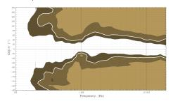
▶ Dispersion angle diagrams of a single A10 in the horizontal plane for all Panflex settings using lines of equal sound pressure at -3 dB, -6 dB, -12 dB.
