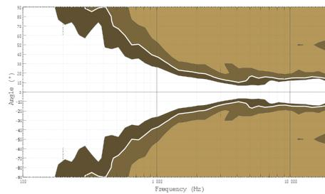
► Dispersion angle diagram of a single A10 Focus (left) and A10 Wide (right) in the vertical plane using lines of equal sound pressure at -3 dB, -6 dB, -12 dB.
