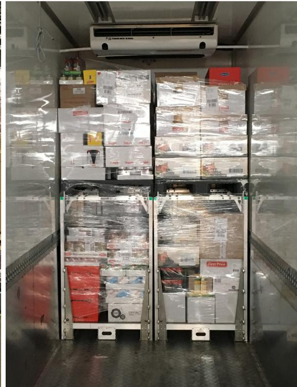
*SpaceInvader doubled-stacked pallet racks lined up in terminal - and in truck before departure. ASKO Hedmark, Central Norway*
