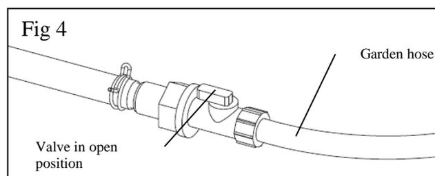
3. Route the garden hose to a sewer drain capable of safely assimilating 1135 plus liters (300 plus gallons) of water which may contain both unsanitary contaminants and chemical residue. Open the drain valve (as shown in Fig 4). The spa drains slowly.
