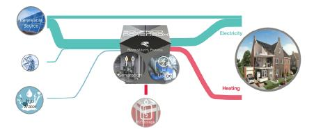
At night or when there is a lack of electricity, the stored hydrogen can be transformed by the reversible PEM fuel cell side into electricity and heat. The electricity goes to appliances and the heat is used for low temperature heating systems as well as sanitary water heating.
