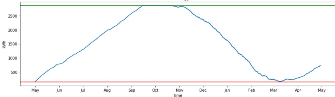
One can see that despite a short period when grid consumption was required during the commissioning of the system (fig. 4, month of May), the installation became self-sufficient. It proves seasonal storage at residential scale by the use of hydrogen storage, supporting the penetration of RESs.
