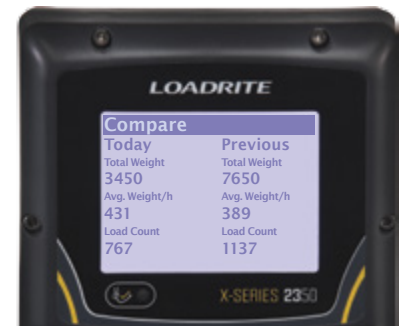
Performance data is stored to allow the operator to compare performance vs. previous, average and best shift
