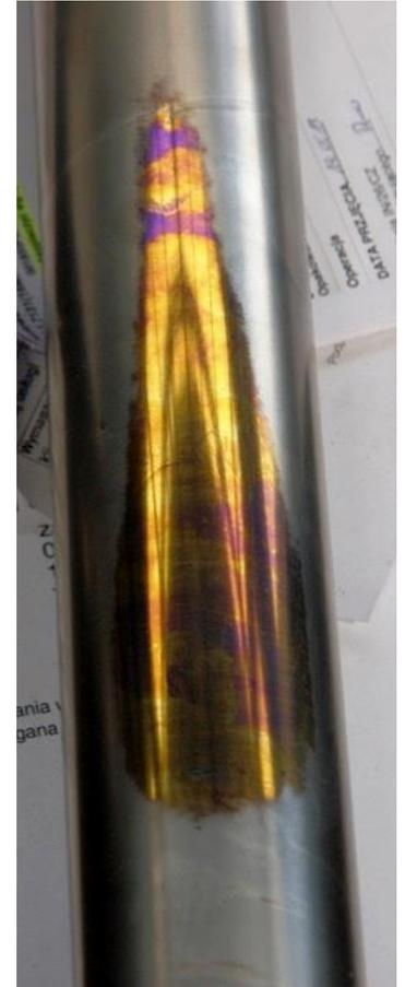
Macroscopic inspection has not revealed large differences in surface quality. Only the hardness measurement has shown significant differences in the effects of nitriding.
