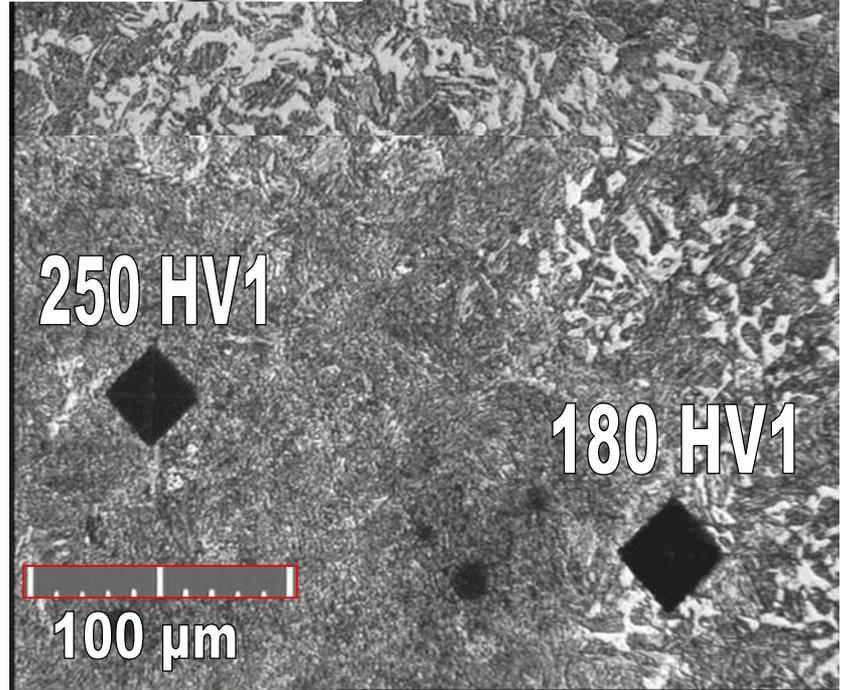
An additional aspect is the microstructure of the raw material, which has a significant impact on cutting parameters.
