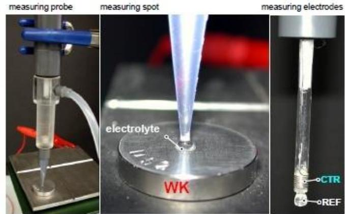
Electrochemical measuring probe
