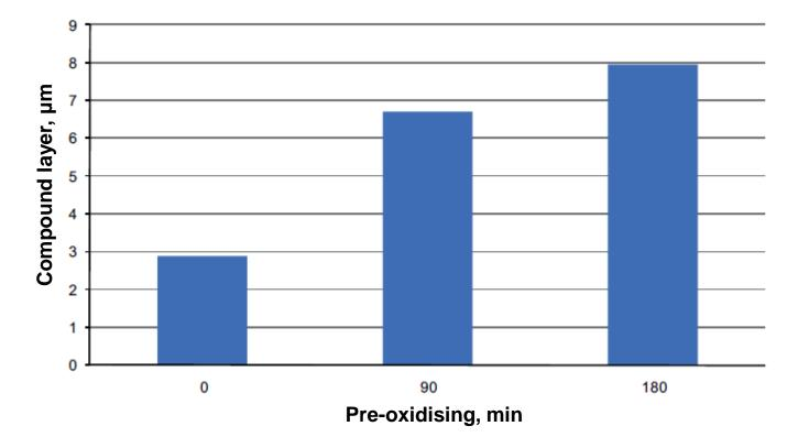
Effect of pre-oxidation on nitrocarburising results. Nitrocarburising 580°C 45min, steel 42CrMo4
