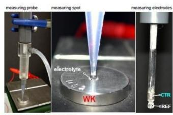
Electrochemical measuring probe
