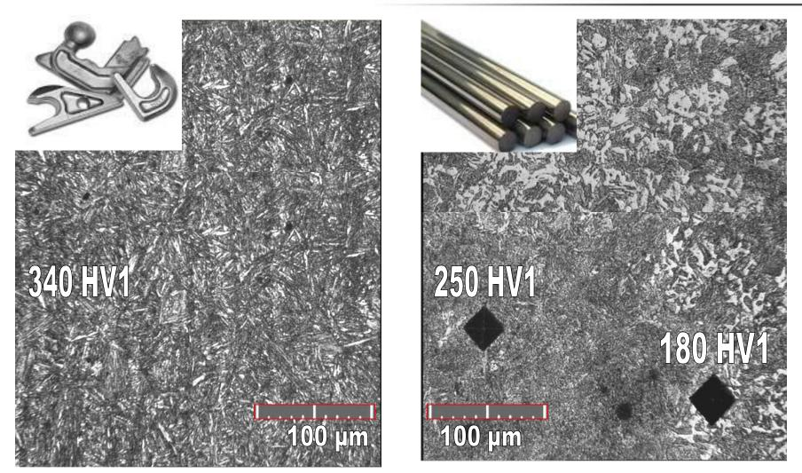
An additional aspect is the microstructure of the raw material, which has a significant impact on cutting parameters.
