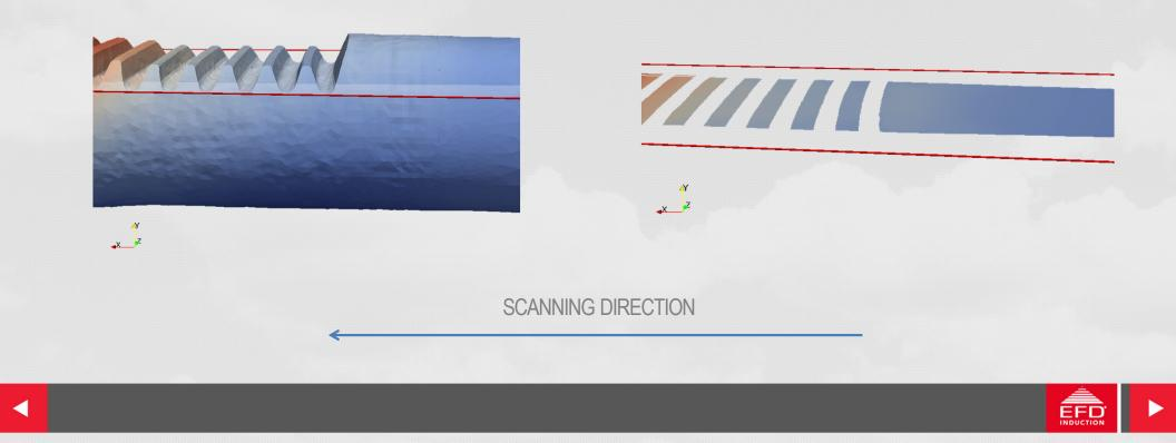
PROBLEM – EXCESSIVE BULGING OF TEETH IN THE CASE OF NO PREHEATING
