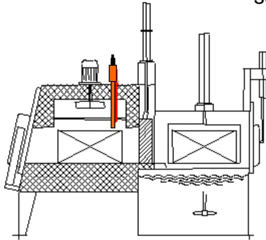
**Bricked sealed Quench Furnace**
