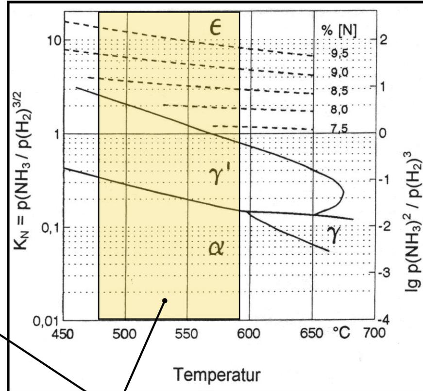
Temperature range normally used for Nitriding or Nitrocarburizing processes
