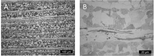
Microstructure as delivered in cross-rolling direction
