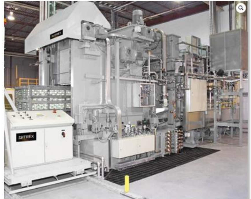
Nitrex multi-chamber furnace for high volume FNC with ONC option.
