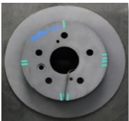
Smart-ONC® coated discs combined with NAO pads
